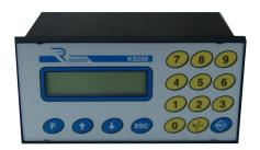
The KS203 is a multi-quota positioner. The selection of the quota to be reached takes place via the keyboard setting (KEY F). When the start is pressed, the instrument automatically performs the quota by acting on the 4 relay outputs. By moving the axis in manual mode the instrument works as a meter and displays the value supplied by the encoder.
