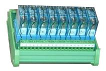
Passive relay interface module that receives digital commands from various electronic devices such as PLCs, industrial PCs, control modules, etc. and controls inductive and resistive loads of small power such as solenoid valves, contactors, small servomotors, lamps, resistors, etc. This type of module has a series of screw terminals that makes it univer-
